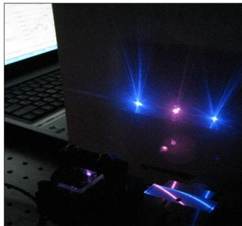
Fig.3. Nonlinear diffraction in the domain structure of SBO.
