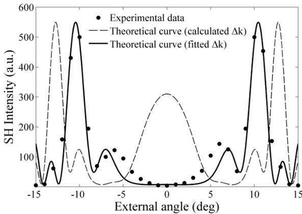
Fig.2. Angular tuning of domain structure for nonlinear optical conversion. (532 nm- $\rightarrow$ 266 nm).
