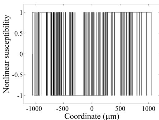
Fig.1. Domain thickness in the sample of SBO.
