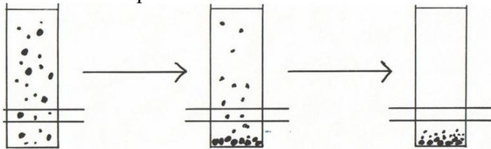
Figure 1 - Integral Sedimentation Method
