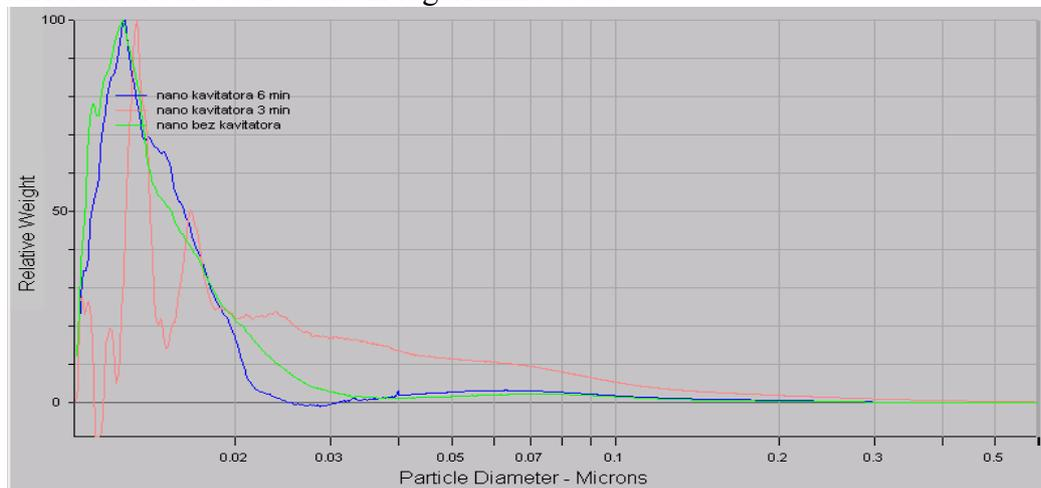
Figure 5. Graphs of distribution of particles mass concentration of a non-dispersed ND suspension (green), 3 minutes dispersion ND (red) and 6 minutes dispersion ND (blue), depending on their sizes
