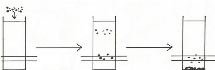
Figure 1. Integral and Differential Sedimentation Method
