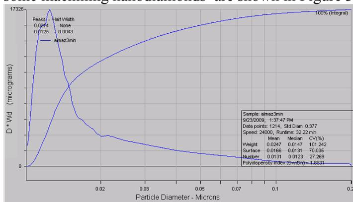
Figure 3. Differential and Integral Distribution of 3 minutes ultrasonic machining ND
