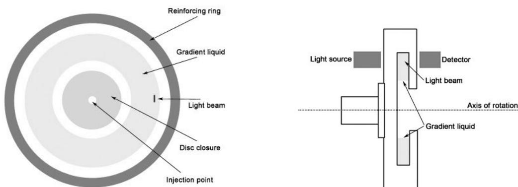
Figure 4 – Hollow Disc Centrifuge Design
