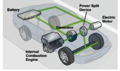
Some of the advanced technologies typically used by hybrids include. Regenerative Braking.
