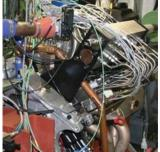
A new hybrid: This prototype hybrid engine, dubbed /4SIGHT, can switch between four- and two-stroke modes, thereby reducing fuel consumption by more than 25 percent.
