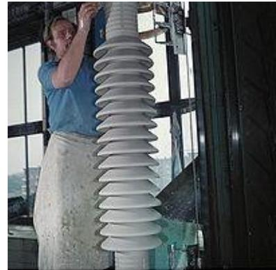
Most high voltage insulators are designed with a lower flashover voltage than puncture voltage, so they will flashover before they puncture, to avoid damage.
