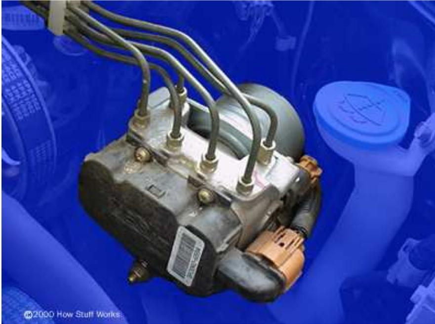
Anti-lock brake pump and valves
