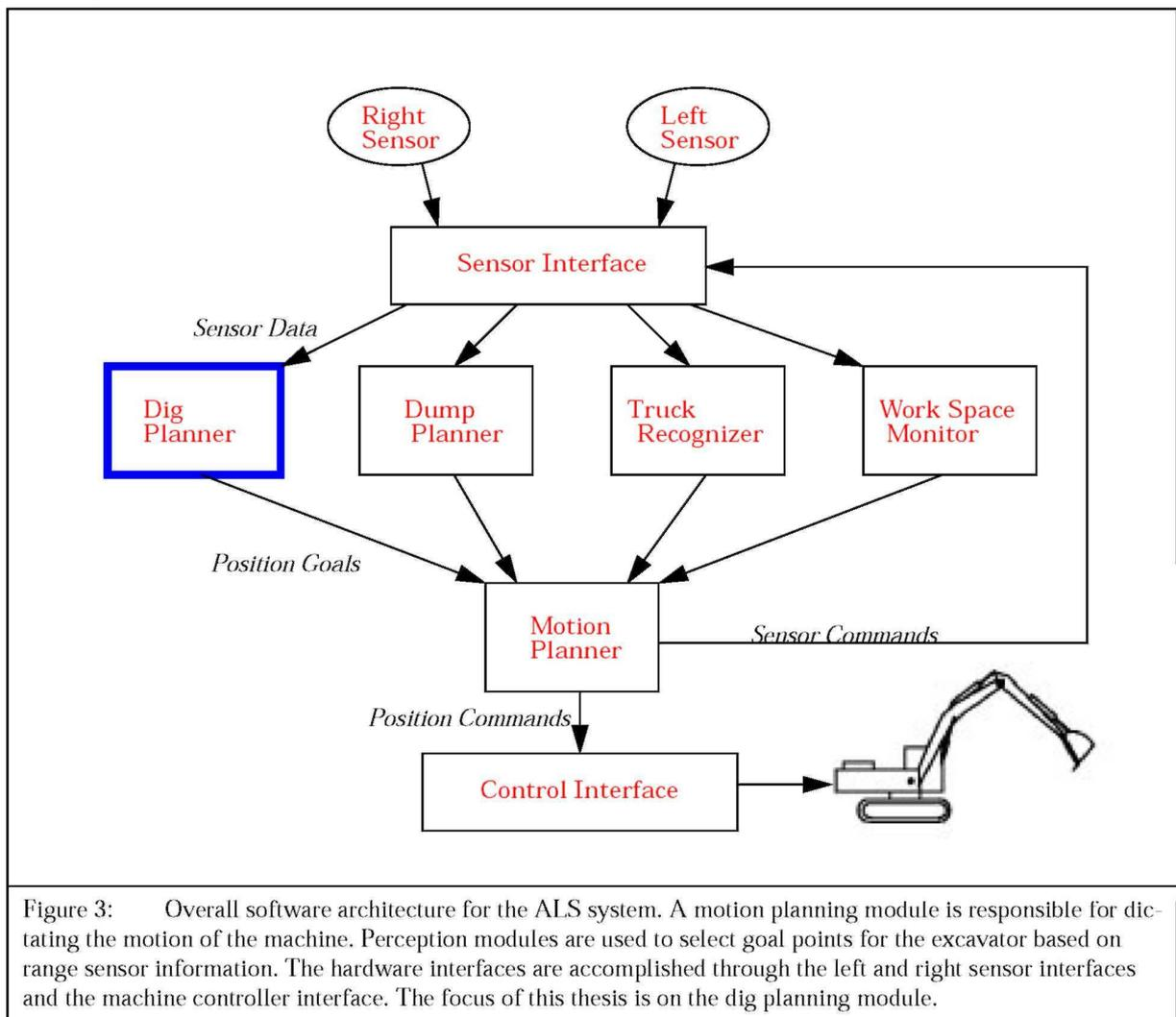
Figure 3: Overall software architecture for the ALS system. A motion planning module is responsible for dictating the motion of the machine. Perception modules are used to select goal points for the excavator based on range sensor information. The hardware interfaces are accomplished through the left and right sensor interfaces and the machine controller interface. The focus of this thesis is on the dig planning module.
