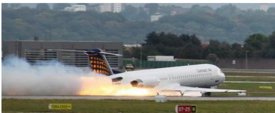
Figure 1 – A passenger jet made an emergency landing on a protective layer of foam
