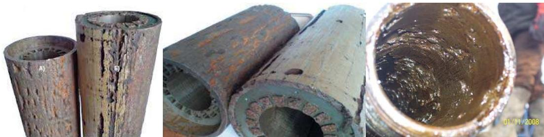
Figure 2 – Corrosion at pipelines
