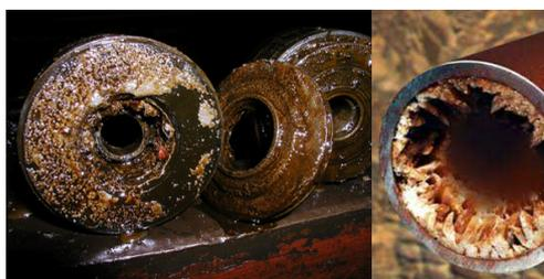
Figure 1 – Salt deposits at pipelines
