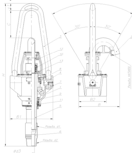
The swivel is a coupling link between tackle system and ancillary. The swivel should retain the drilling string hanged to it and to amortize at its sharp moves and to smooth out its hitches at trippings. And consequently it is responsible drilling equipment in respect of reliability. The swivel must to provide drilling tool trouble-free work, and also safety of servicers.
