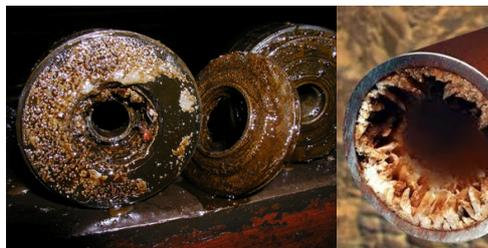
Figure 1 – Salt deposits at pipelines
