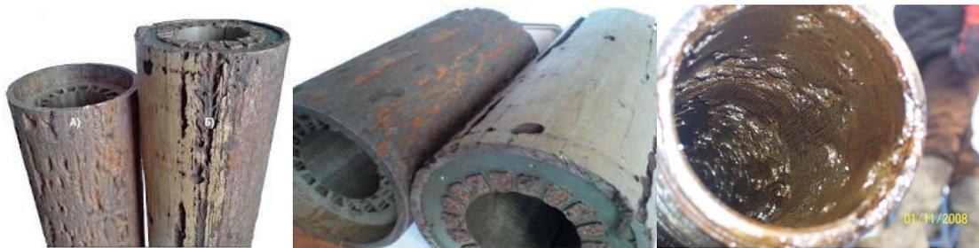
Figure 2 – Corrosion at pipelines
