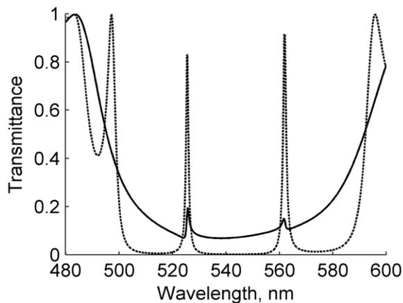
Fig.6. Forbidden zone in the transmission spectrum of the structure. The dotted line - the left polarization. Solid line - right polarization.
